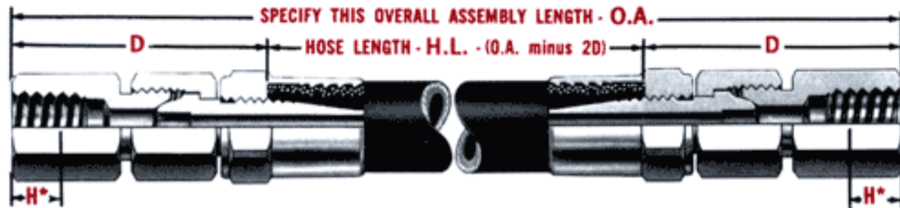
SHOWN ABOVE - EL and SEL ASSEMBLIES THROUGH 3/4" I.D. HOSE SIZE (BRASS FITTINGS)
