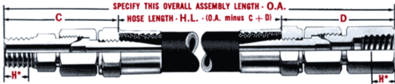
SHOWN ABOVE - FL and SFL ASSEMBLIES THROUGH 3/8" I.D. HOSE SIZE (BRASS FITTINGS)
