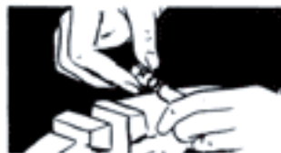
1. Place Ferrule Over Hose End and oil inside of hose.
