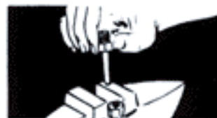
2. Oil stem thread and place stem in Ferrule
